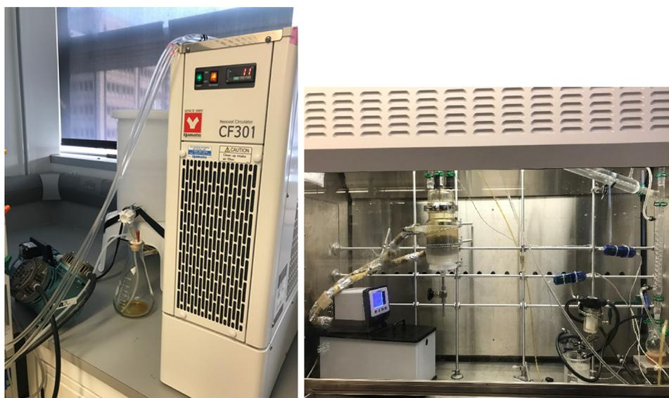
a) the vacuum pump, cooling system and feed tank b) principal part of reclaimer
