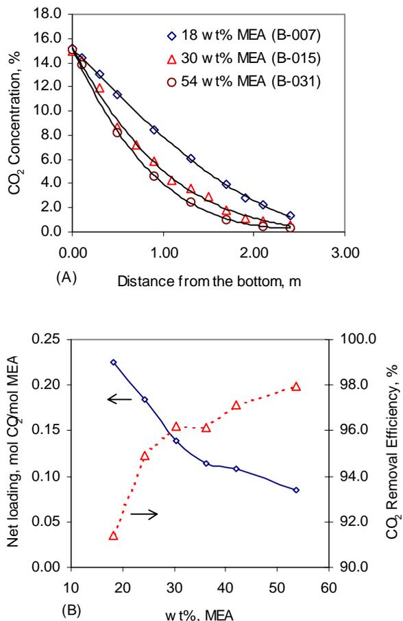
Figure. 1 Effect of absorbent concentration within the range of 18 to 54 wt%. Runs number are: B-007, B014, B015, B-026, B-029, and B-031.
