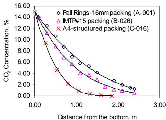
Figure 3. Effect of packing type on the removal efficiency of CO<sub>2</sub>. Runs number: A-001, B-026, and C-016.
