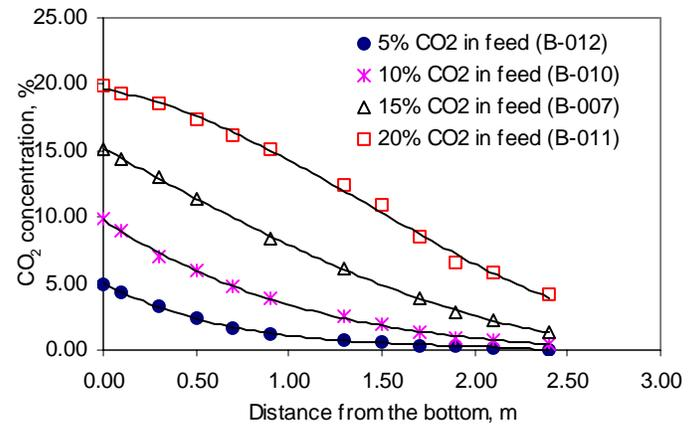
Figure 6. Effect of gas CO<sub>2</sub> concentration on the absorption rate.
