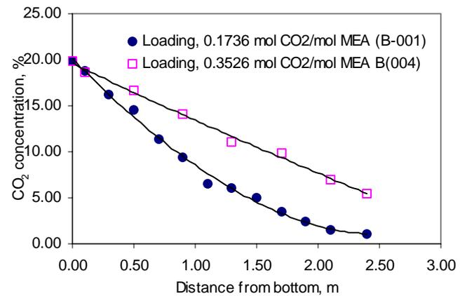
Figure 7. Effect of CO<sub>2</sub> loading on the absorption process
