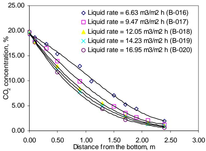
Figure 4. Effect of liquid flow rate on CO<sub>2</sub> absorption into MEA solutions.
