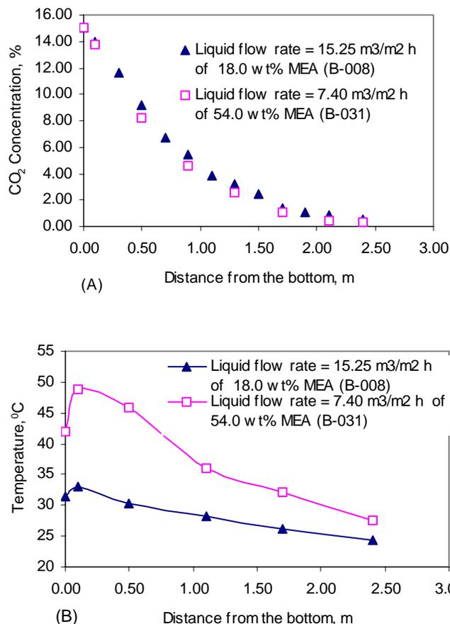
Figure 2. The effect of absorbing the same quantity of CO<sub>2</sub> in a smaller volume of solution on the temperature profile. Runs number: B-008 and B-031.
