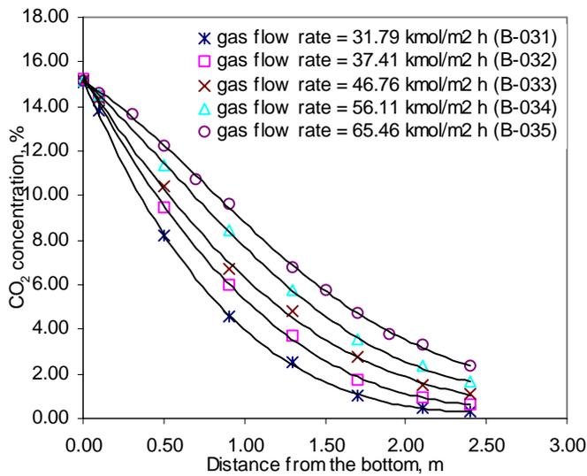
Figure 5. Effect of gas flow rate on the CO<sub>2</sub> absorption
